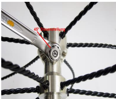
Screwed in nozzles, position 45°
