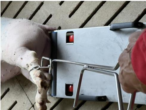
Transporker is stopped with one foot and the user pulls the cadaver onto the platform over the pick-up rollers integrated in the ramp. Using the pull rod, Transporker with the cadaver can now be pulled to the cadaver disposal site.
